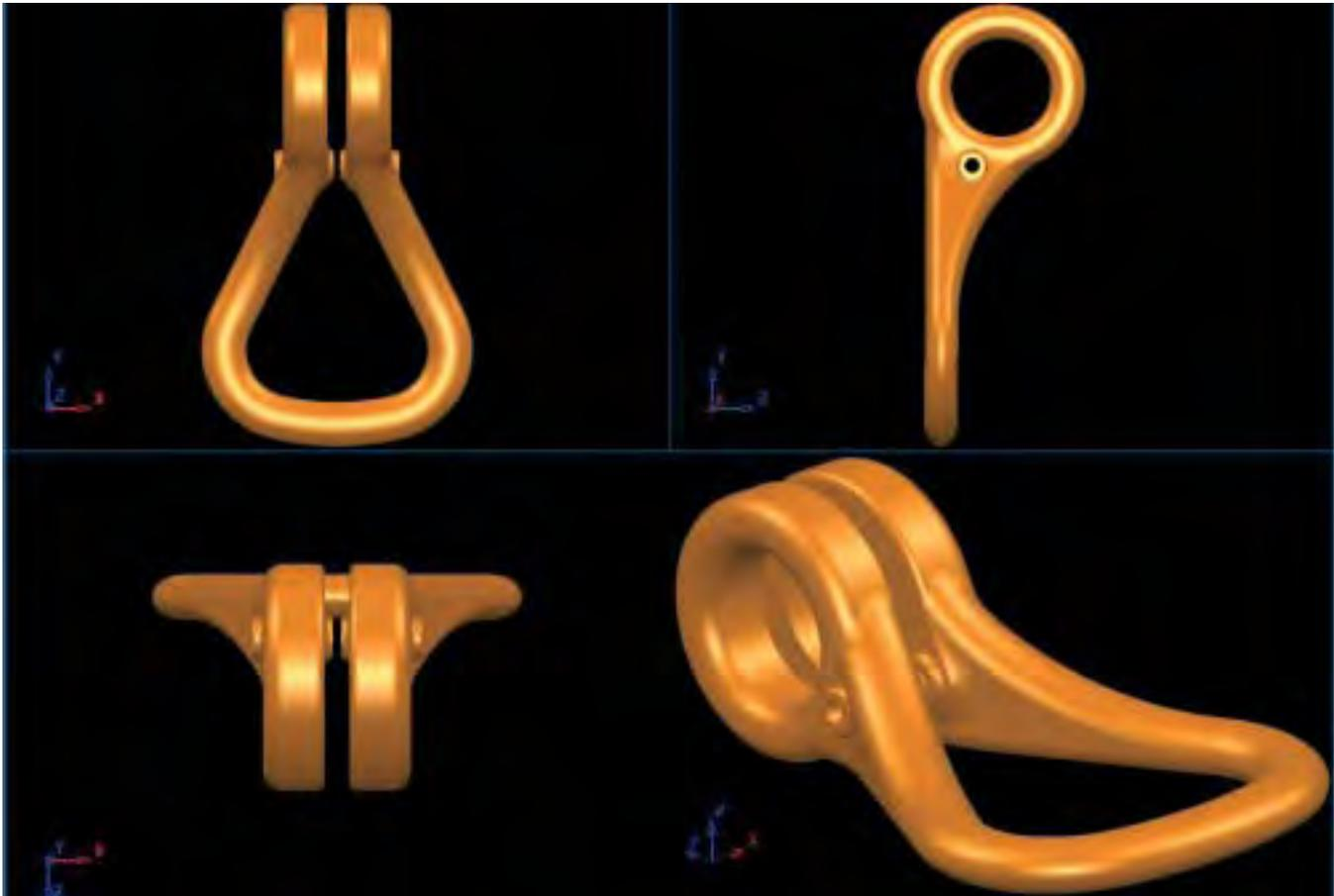
*3D diagram of the new bottom eyelet made of polyamide.*
