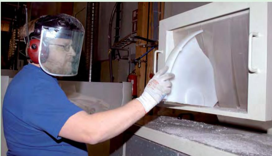
*Molding Master Harri Helin is feeding plastic remnants into the grinder. Tens of tons per year.*
