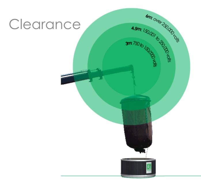
As the waste is collected, the reusable bag and lifting arm must at all times be a safe distance from nearby electrical sources. This may include overhead wires, lights, etc. This diagram shows the safe distances by voltage.
