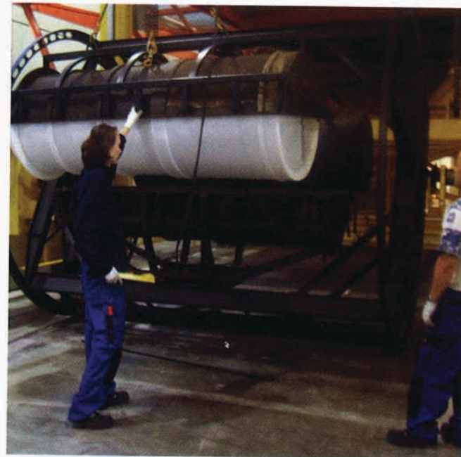
A new Molok is born. This multi-million-dollar German machine transforms molds containing flaked polyethylene into various shapes and sizes of Moloks using heat and rotation.
